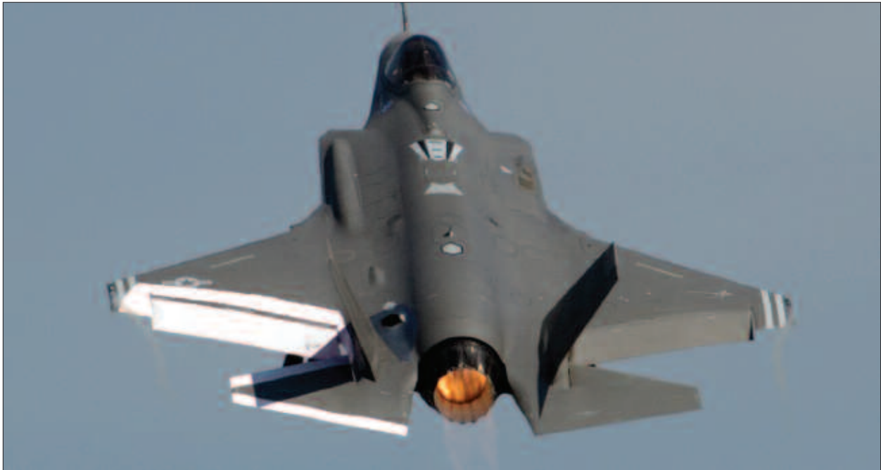
Because the Joint Strike Fighter is a single-engine aircraft, each engine must be extremely reliable to guarantee the safety of pilot and plane.
